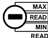
To read the Maximum or Minimum INPUT since READ mode was entered, simply switch to MAX or MIN. The value will appear on the LCD along with the word MAX or MIN. The MAX/MIN values are automatically updated and may be viewed at any time without disturbing the other values.
