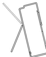
The Model 434 comes with a carrying case and a built-in tilt stand/hanger. The 434 is held securely in the case by VELCRO®.
